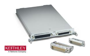
The 7709 plug-in module is a two-pole, 6×8 matrix module. It can connect any combination of six differential channels of instrumentation to any combination of eight differential deviceunder-test channels. The instrumentation can be AC and DC sources, internal or external meters, oscilloscopes, etc. This matrix configuration allows wide flexibility for complex test systems.
