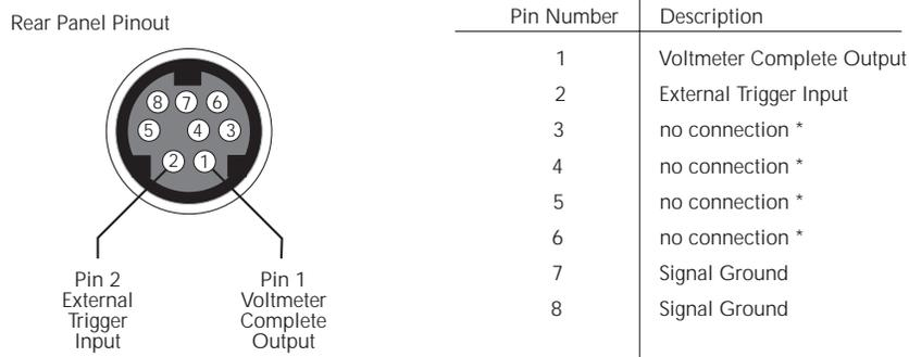
\* Either pin 3 or 5 may be configured as an output instead of pin 1. Either pin 4 or 6 may be configured as an input instead of pin 2. See the optional Model 2000 Repair Manual for details.
